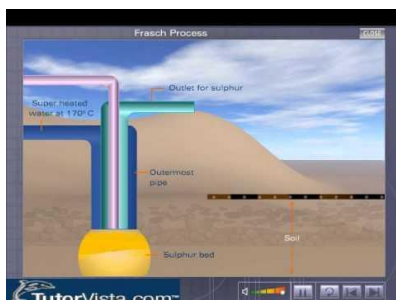
frasch process of sulphur extraction
