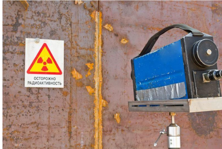
An industrial radiography camera being used to inspect a weld for defects
